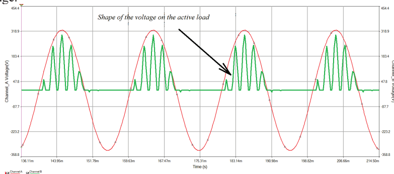
Fig.5. Shape of the voltage on the active load without the low-frequency LC filter
