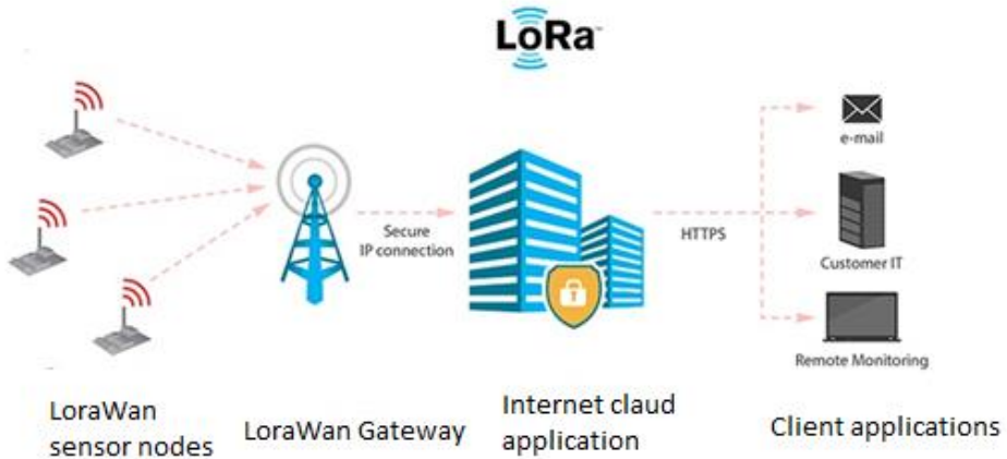
Fig.1 Architecture of LoraWan measurement systems for temperature and relative humidity
