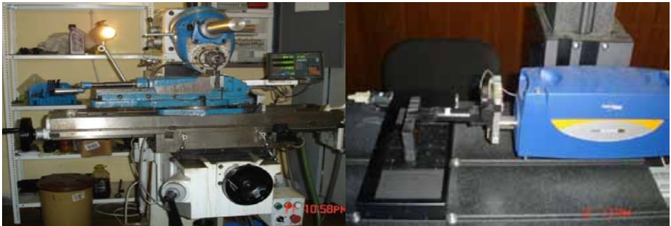
Fig. 5.1. Machine with which it is made the Fig. 5.5. Measuring device for measuring the realization of the sample preparation severity of the processed surface TALYSURF (FATS-Mitrovica). - Intra (FATS-Mitrovica)
