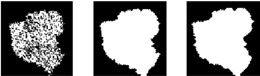
Fig. 2. Originally segmented image, dilated image, eroded image (from left to right).
