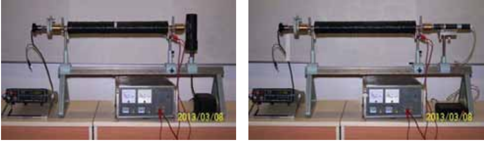
Fig. 2: Photo of the experimental setup: left – with calibration sodium lamp, right – with a laser.
